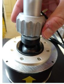
\*Note: Some bases, including the Thrustmaster Warthog, will not be properly recognized by Windows if the original manufacturer's grip is not installed on the base the first time it is plugged into your PC. Once you have connected the base (with original grip) into your PC an installed all necessary drivers, you may remove the OEM grip and install the SopGrip without issue.
