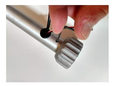
Once the screw is disengaged, slide the mounting adapter out of the control column, and remove the old locking nut. Re-assembly is the reverse of removal.
